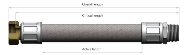
**Critical length** is the distance between hose mating faces. This must be 10% greater than the actual distance between the two corresponding fixed mating parts to avoid tensile stress whilst in service.
